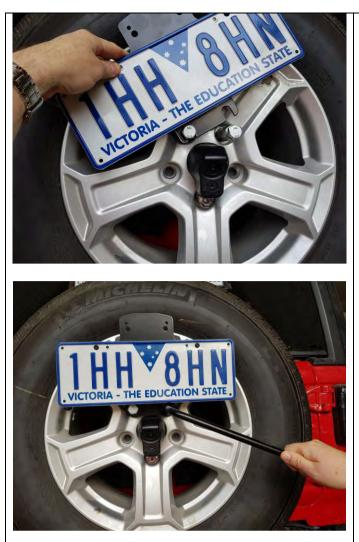
14. Fit the plate onto the bolt shank as shown. Then use the wheel brace to tighten the bolts up securing the plate. ..
